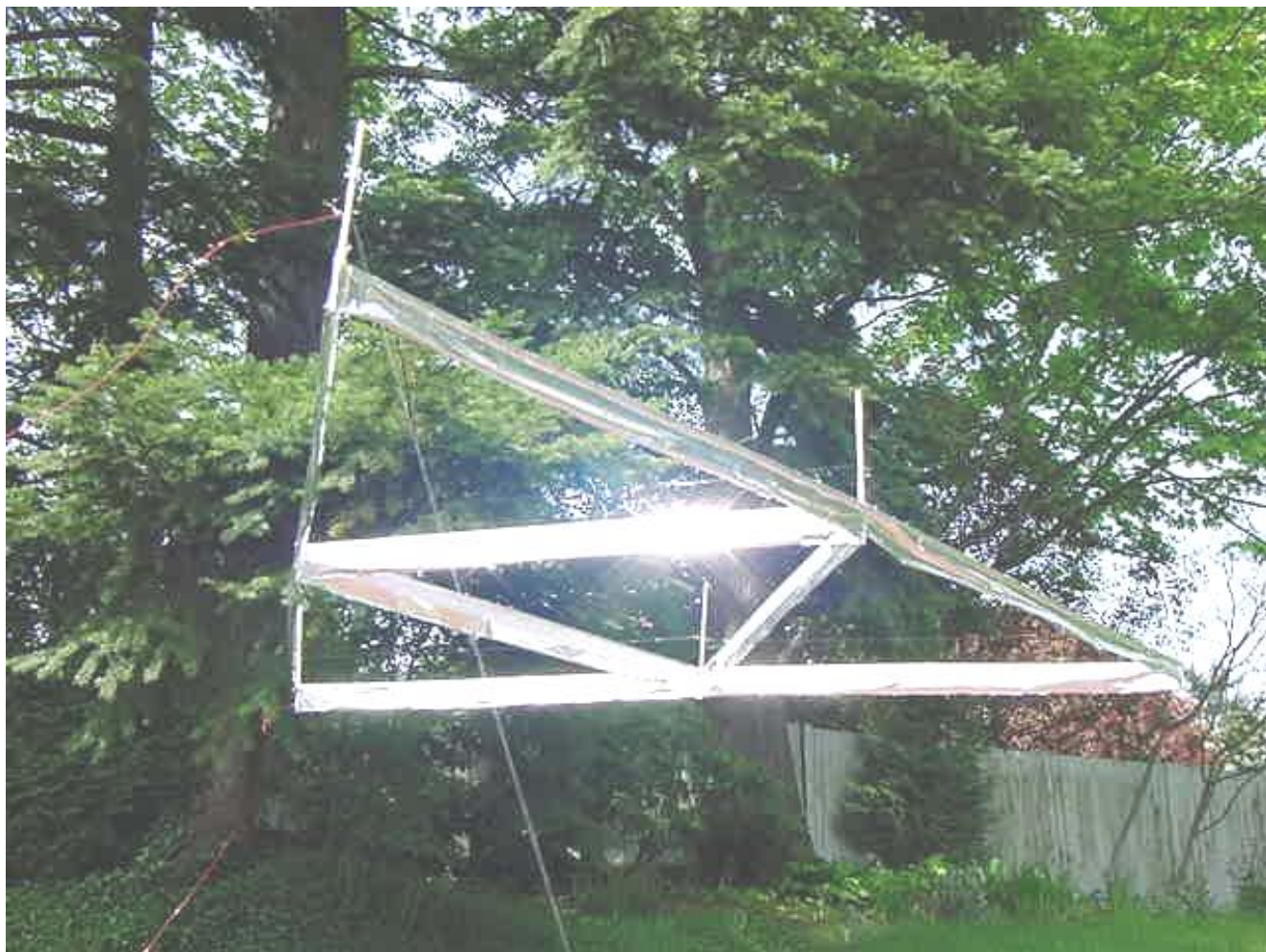
Figure 92 - photo of "Lifter" (Biefeld-Brown Effect) (courtesy Tim Ventura, May 2002)
