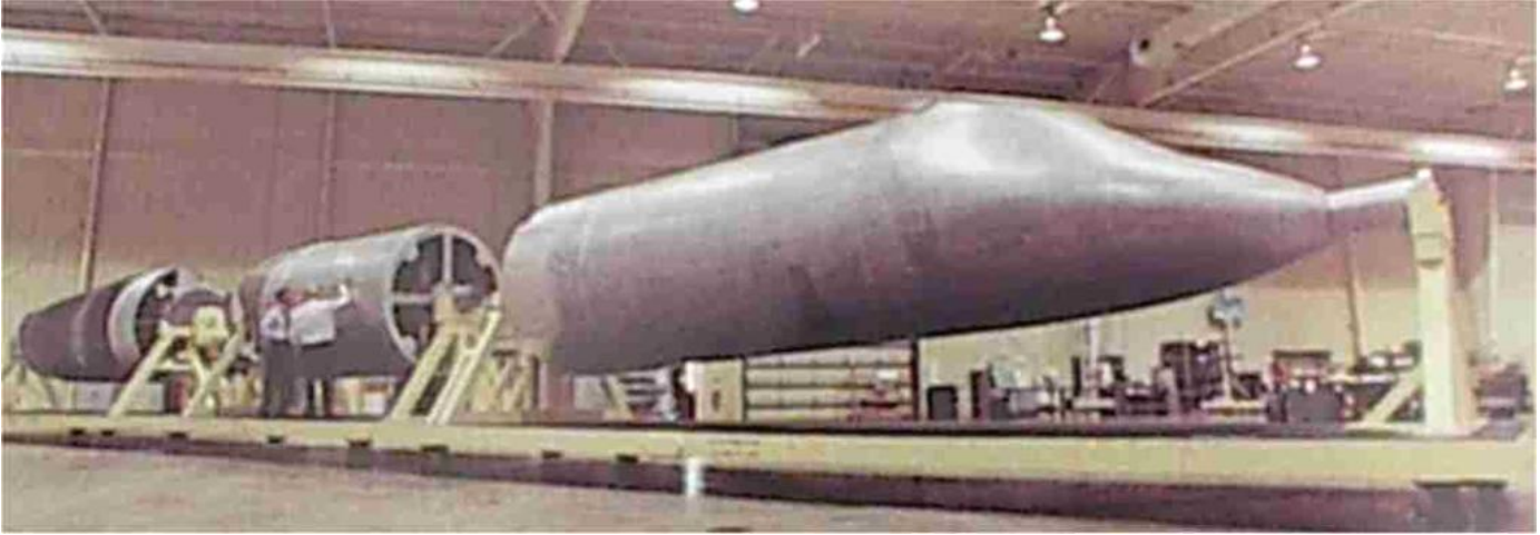
Figure 27 - Fuselage Mandrels at Cincinnati Machine's plant
