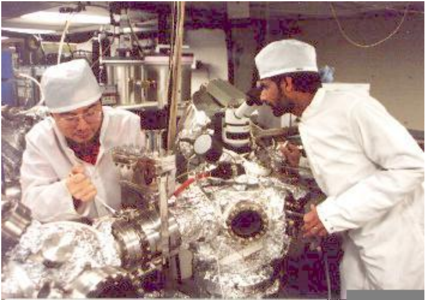
Figure 55 - Dr. Sivananthan (Director/UIC Microphysics Labs) and co-worker using MBE equipment that will be used in producing UNITEL's lens
